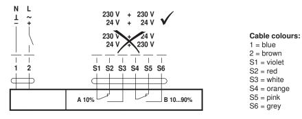
Rotary spring-return actuator, Open-close, AC 24...240 V / DC 24...125 V, 20 Nm, with 2 integrated auxiliary switches
