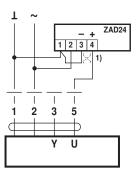
Control with 4...20 mA via external resistor
