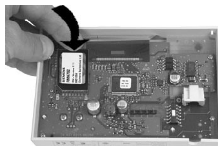
Fitting the memory card
