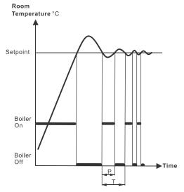
In general, PID control provides more comfort and is more energy efficient than 2-position control.
