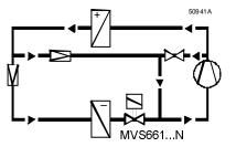
Typical control range 10...100 %. The capacity controller ensures that the compressor is adequately cooled, making it unnecessary to set a minimum stroke in the refrigerant valve.
