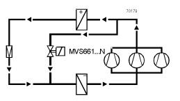
Suitable for use in large refrigeration systems in air conditioning plant, to prevent unacceptable temperature fluctuations between the compressor stages.
