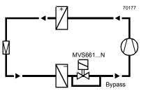
Typical control range 50...100 %. Minimum stroke limit control: To ensure optimum cooling of the compressor, either a capacity controller must be provided for the compressor, or a minimum stroke must be set via the valve electronics.
