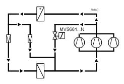
Suitable for large refrigeration systems on air conditioning applications with several compressors or compressor stages, and where the evaporator and compressor are some distance apart (attention must be paid to the oil return).
