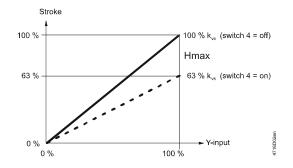
When  $k_{vs}$  reduction (DIL switch 4 in position ON) the stroke will be limited to 63 % mechanical stroke. 63 % of full stroke then corresponds to an input / output signal of 10 V. If, in addition, the stroke is limited to 80 %, for example, the minimum stroke will be
