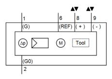
Tool = Configuration and maintenance interface (7-pin)
