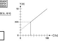
Control with 4...20 mA via external resistor
