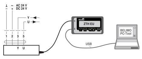
Linear actuator, parameterisable, modulating, AC/DC 24 V, 200 N, Running time motor 7 s
