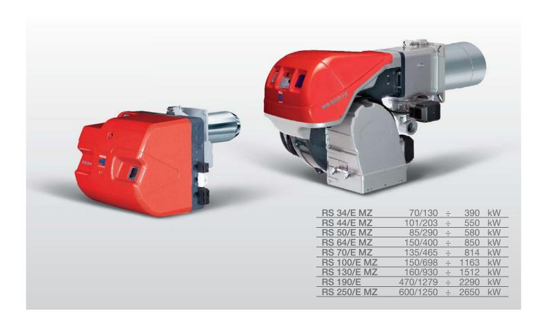
The RS/E MZ burners series covers a firing range from 70 to 2650 kW, and it is based on a new Digital Burner Management System, Riello REC27, which is able to manage the air-fuel ratio by independent servomotors in order to obtain a perfect output control and to assure a correct combustion and safe operation on all modulation range.
