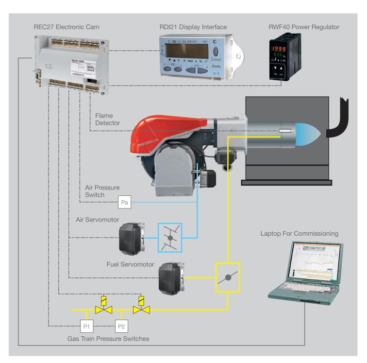
REC27.100A2 Digital Burner Management System Layout.
