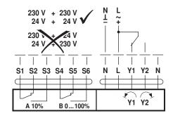
AC 24...240 V / DC 24...125 V, 3-point, Auxiliary switches
