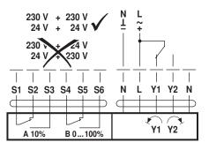
Rotary actuator, Open-close, 3-point, AC 24...240 V / DC 24...125 V, 160 Nm, Running time motor 35 s
