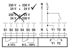
AC 24...240 V / DC 24...125 V, 3-point, Auxiliary switches
