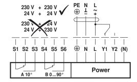
AC 24...240 V / DC 24...125 V, 3-point, Auxiliary switches
