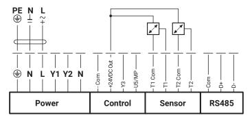
Switching contact connection (BACnet MS/TP / Modbus RTU)
