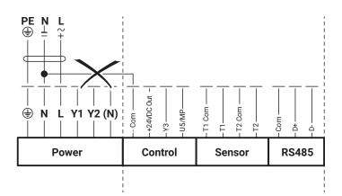
Power supply must not be connected to the signal terminals!
