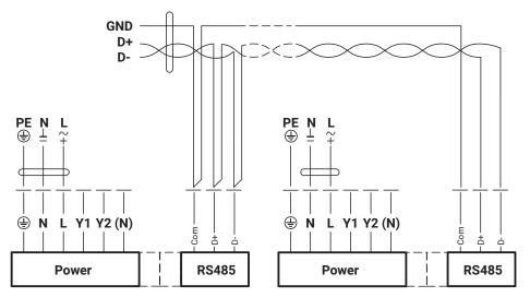
Connection BACnet MS/TP / Modbus RTU with analog setpoint (hybrid mode)
