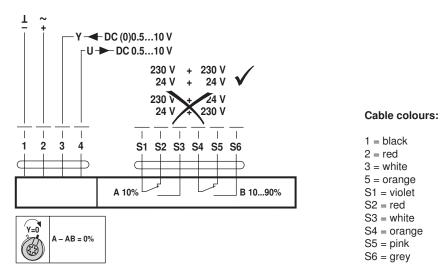
Rotary spring-return actuator, Modulating, AC/DC 24 V, 10 Nm, with 2 integrated auxiliary switches
