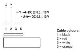
Override control (frost protection circuit)
