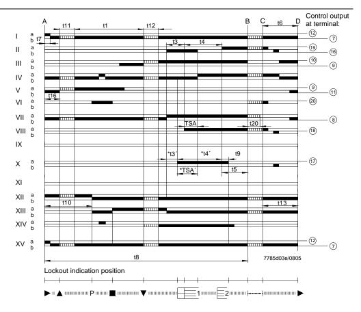
\* Times TSA', t3' and t4' are only programmed by burner controls LGK16.335... and LGK16.635...
