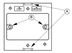
Mark the position of the holes (B) on the wall and drill holes 5 mm in diameter. Insert plastic plugs into holes.
