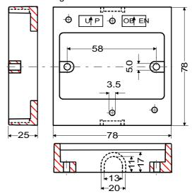
Figure 2: TM-1100-8931 Surface Mounting Kit
