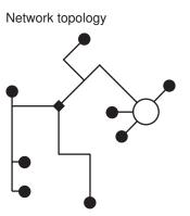
There are no restrictions for the network topology (star, ring, tree or mixed forms are permitted). Supply and communication in one and the same 3-wire cable • no shielding or twisting necessary
