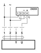
Control with 4...20 mA via external resistor
