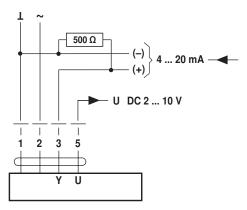
The 500 Ohm resistor converts the 4 ... 20 mA current signal to a voltage signal DC 2 ... 10V
