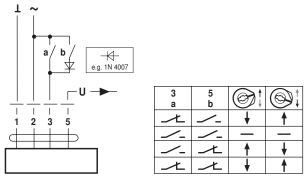
Functions when operated on MP bus
