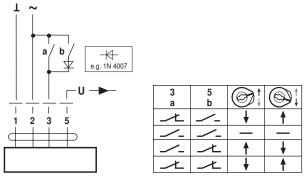
Functions when operated on MP bus
