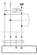
Supply and communication in one and the same 3-wire cable • no shielding or twisting required • no terminating resister required
