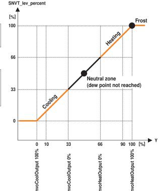
Heating / cooling with Belimo 6-way characterised control valve.
