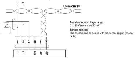
Actuator for LONWORKS®, AC/DC 24 V
