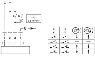
Functions when operated on MP bus
