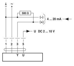
The 500  $\Omega$  resistor converts the 4 ... 20 mA current signal to a voltage signal DC 2 ... 10 V
