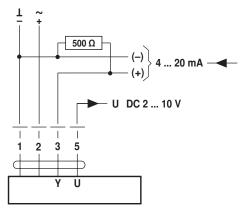
The 500  $\Omega$  resistor converts the 4 ... 20 mA current signal to a voltage signal DC 2 ... 10 V
